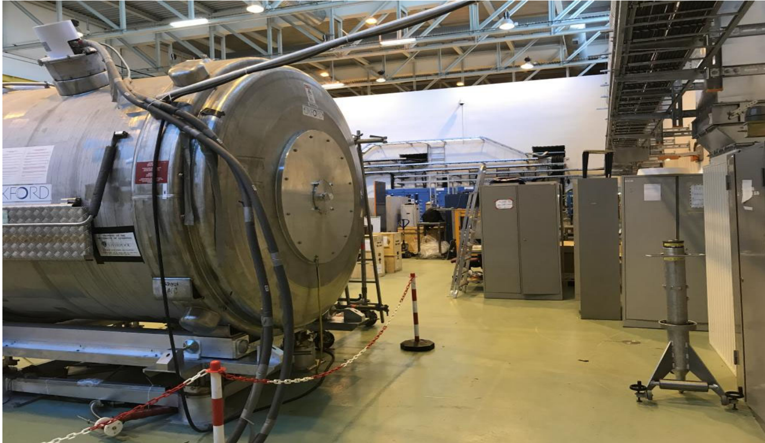
Usual MRI magnet from a hospital (after some refurbishing)
